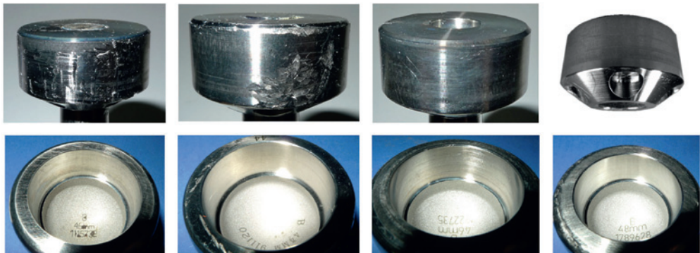
Figure 6. Representative examples of the male (outer) adapter tapers (top row) and the corresponding female head tapers (bottom row). Most adapter tapers exhibited serious disassembly marks which did not allow surface analysis.
