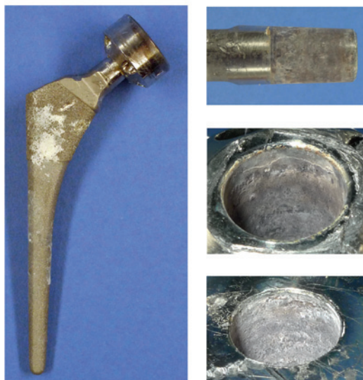
Figure 4. Example for an adapter still connected to the stem after revision (left). After disassembly, severe corrosion was visible on the stem taper and the female adapter taper (right). The distal part of the female adapter taper (middle right) showed thicker oxide layers than the proximal part (bottom right).
